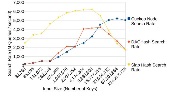
Results from an experiment where 2<sup>25</sup> elements were searched for in the table across varying input sizes. Same configuration as before except bucket count is 2<sup>20</sup> for all tables.
